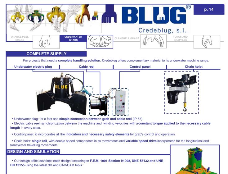
• Each new design is validated and optimised using **Finite Elements Analysis** technique in the way to analyse fatigue effects and warranty **2.000.000 cycles** for components' and machines' working life.
